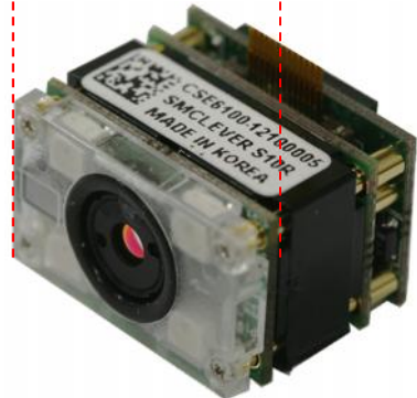
Our Engine with Decoder [20(W)*12.5(H)*17.5(D) mm]
